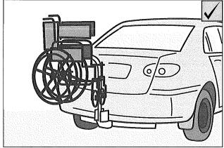
Wheelchair carriers mounted to the tow bar of a vehicle reduces lifting and reaching for the worker.
